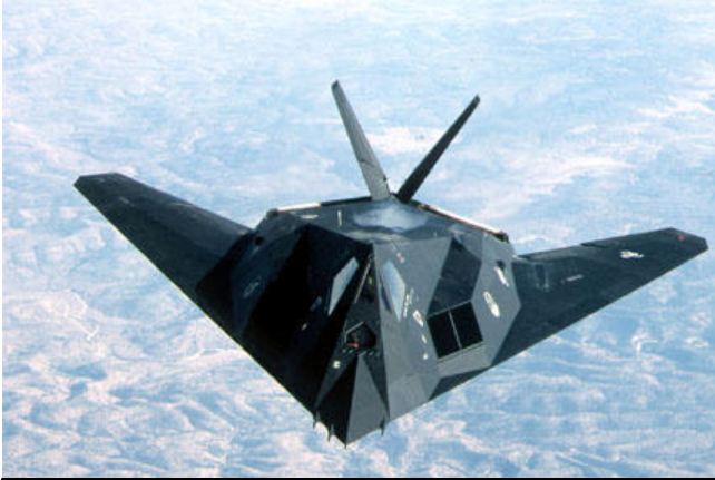
Figure 4 - F-117 Nighthawk Stealth Fighter (Note the faceted shape – there are very few curved edges on the aircraft's exterior.)
